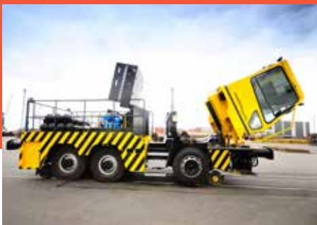
Easy access for maintenance
